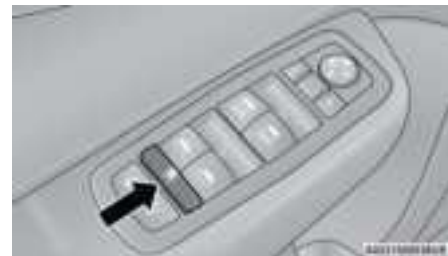
Window Lockout Switch
