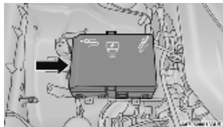
Front Power Distribution Center
