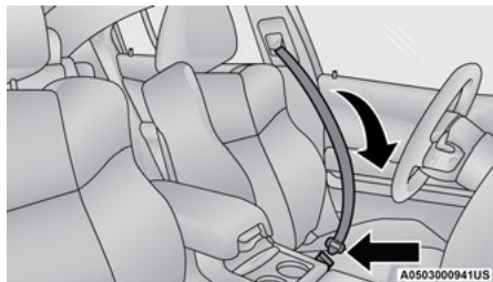
Pulling Out The Latch Plate
