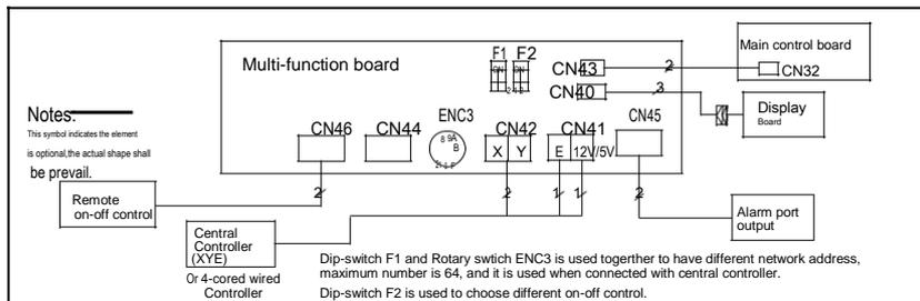
Note: Shielded cables must be used to connect with 4-cored wired controller and central controller. The length of the cables should not exceed 50m(164ft).
