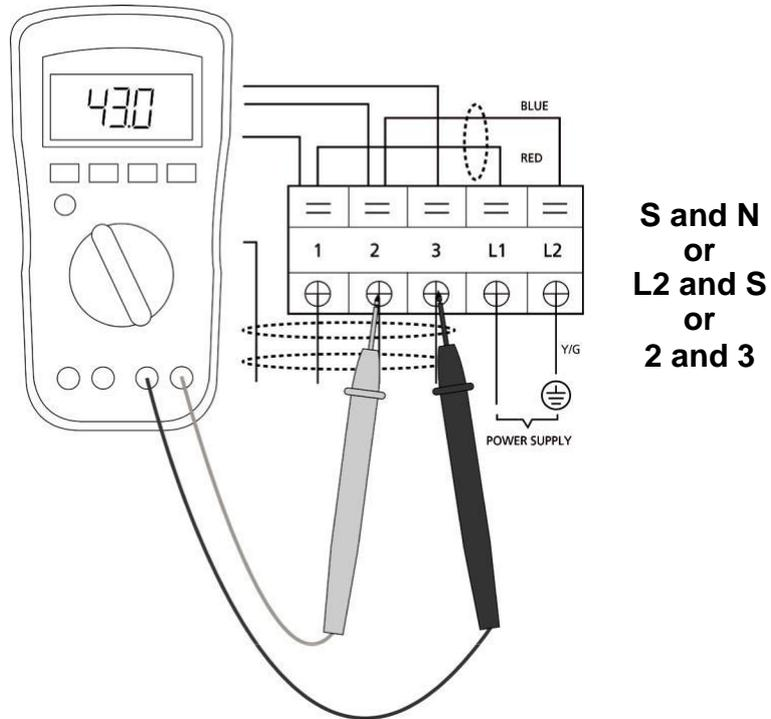
Use a multimeter to test the resistance of the reactor which does not connect with capacitor. The normal value should be around zero ohm. Otherwise, the reactor must have malfunction.
