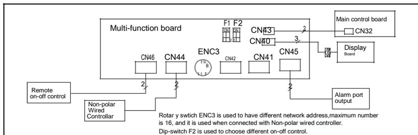
Note: Shielded cables must be used to connect with non-polar wired controller. The length of the cables should not exceed 50m(164ft).
