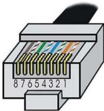
Figure 4.2 Pin Configuration of Type T-568B RJ45 Plug
