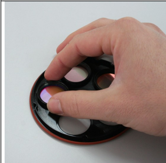
Install filters on disk
