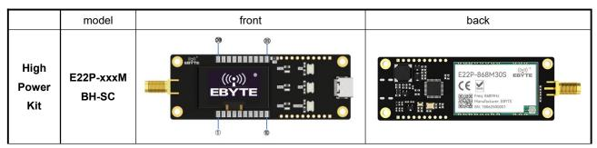
The SC Series Evaluation Kit is designed to help users quickly evaluate Ebyte's next-generation footprint-compatible wireless modules. The MCU uses the STM32F103C8T6, and all available pins are broken out to two pin headers. Developers can easily connect a variety of peripherals using jumpers, facilitating secondary development.
