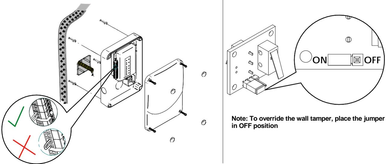
**Note: Follow the same connection model, using the CU tamper input, when using a third party electric box equipped with a tamper opening detection.**
