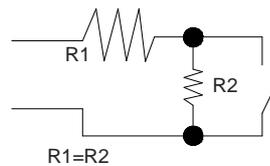
The resistance value R1 and R2 are defined in the software: 1k (recommended), 1k5, 2k2, 3k3, 4k7, 6k8, 10k
