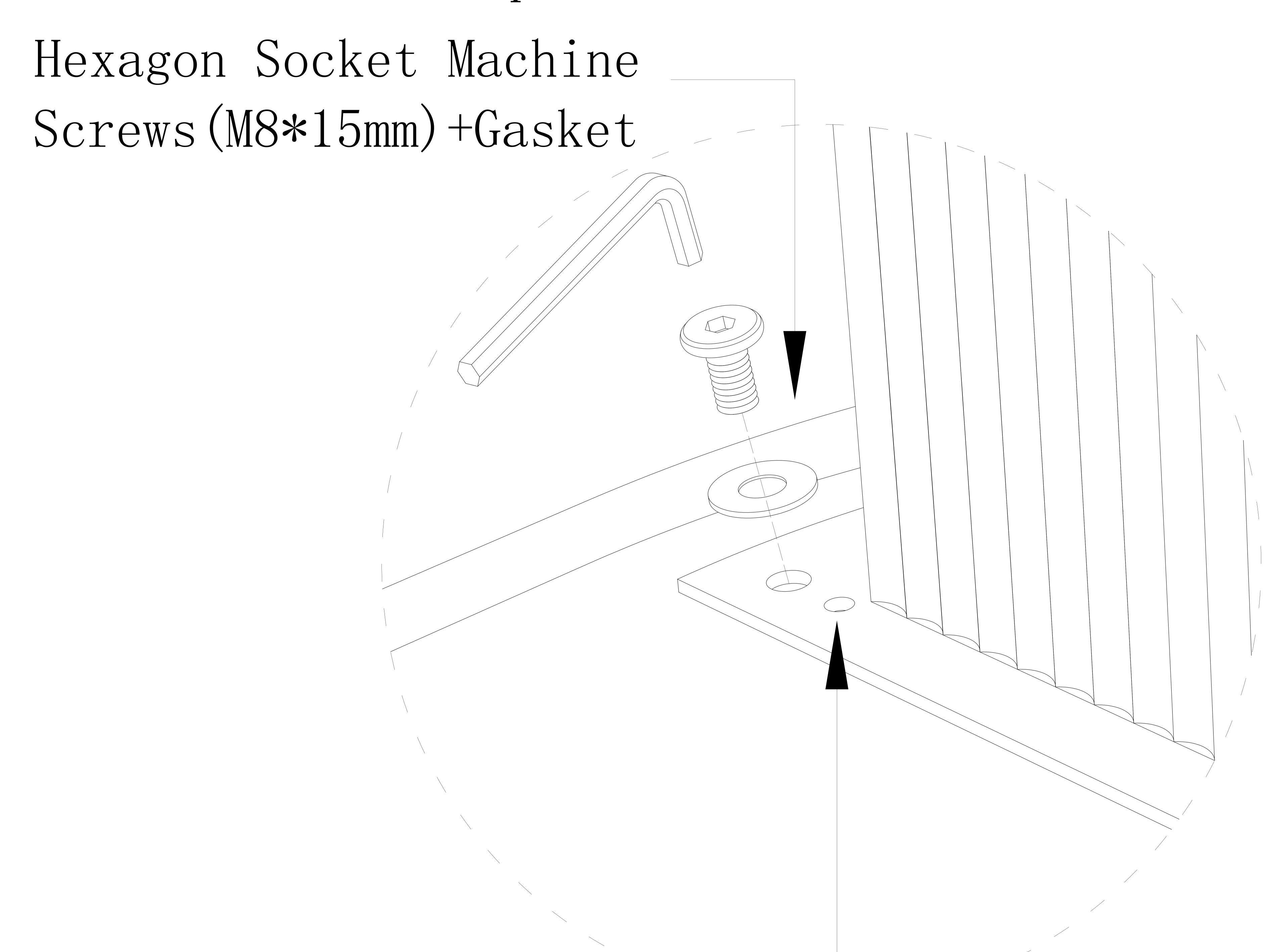
Spare Holes (Hexagon socket machine screws holes can be screwed into the use of Self-drilling screw when damaged)
