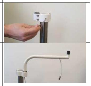
3. Insert the cable through the small opening of the fixing bracket and place the angular arm in it.
