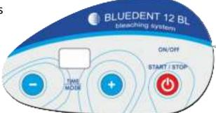
7. To Stop the bleaching device at any time press the START / STOP button. If the device is not manually stopped it will stop after the selected time has elapsed. Note that the fan will continue to work for some time in order to cool down the unit.
