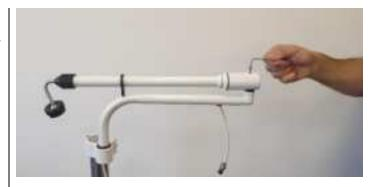
5. Altering the force required to move the straight arm up and down is done by adjusting the screw (located on the back of the central position locking mechanism) with a 5 mm Allen key (included in the package).
