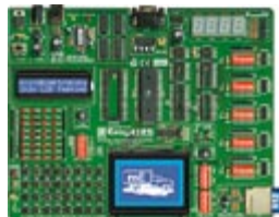
EasyAVR5 Development Board with on-board USB 2.0 programmer
