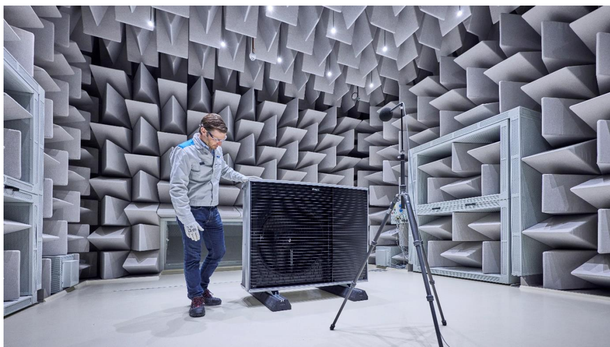
Daikin Altherma 4 H air-to-water heat pump brought to test at in-house acoustic laboratories
