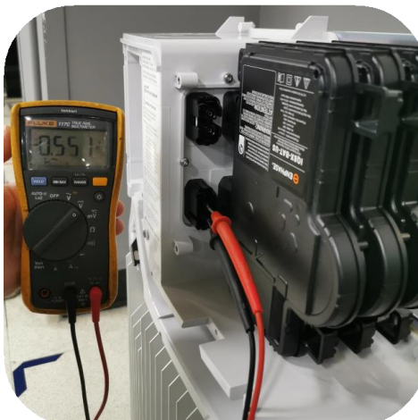
Figure 7: DC Measurement must be below 1 Vdc before connecting IQ8X-BAT NB microinverter
