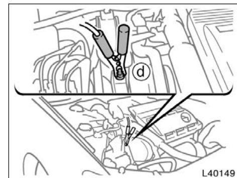
Connecting point for 1MZ-FE and 3MZ-FE engines
