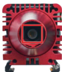
**EN** If the laser module is not used for a long time or is used for more than 30 hours, clean the lens with medical alcohol and cotton swab. Unclean lenses can weaken the power of the laser .
