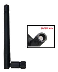
Figure 2: LoRa Antenna
