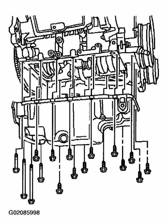
Fig. 250: Installing Oil Pan Bolts
