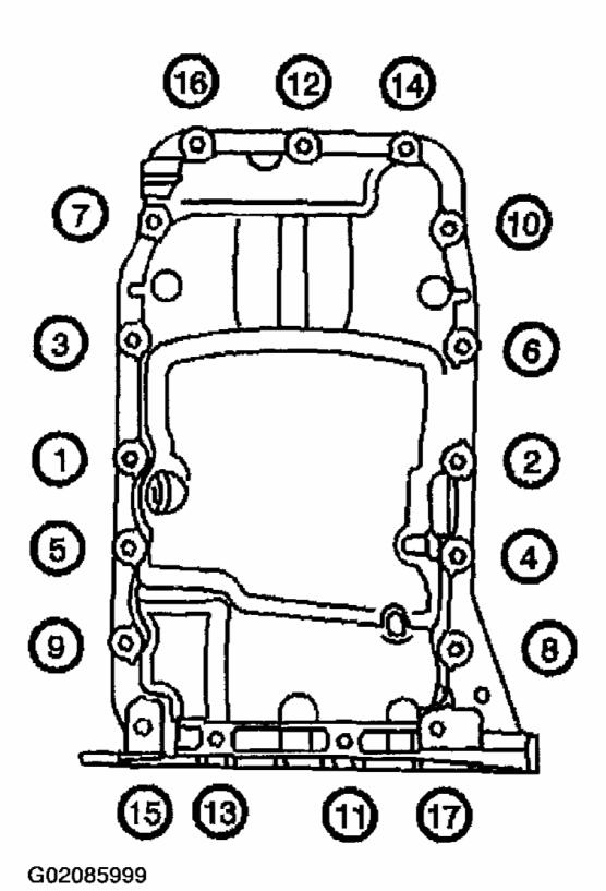
Fig. 251: Identifying Oil Pan Bolt Tightening Sequence
