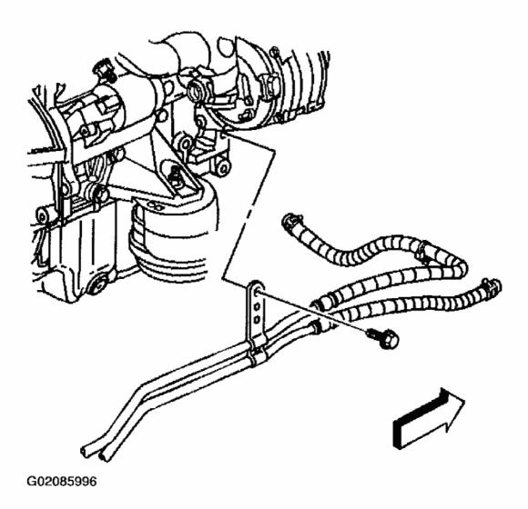
Fig. 248: Removing Transmission Fluid Cooler Pipes Brace Bolt Courtesy of GENERAL MOTORS CORP.
