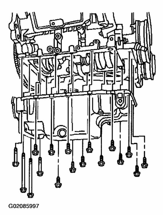
Fig. 249: Removing Oil Pan Bolts
