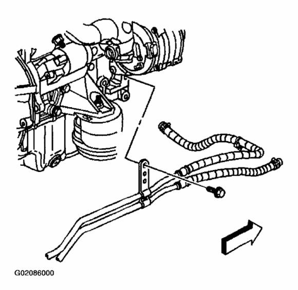
Fig. 252: Installing Transmission Fluid Cooler Pipes Brace Bolt Courtesy of GENERAL MOTORS CORP.
