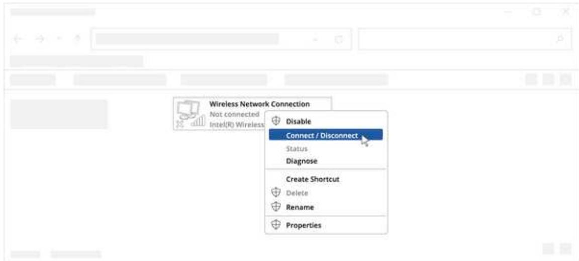
5. Choose the wireless network RUT241 \*\*\*\* from the list and click Connect. Enter the Wi-Fi password located on the device's label.
