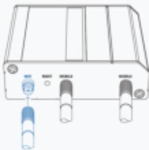
7. Connect the 4-pin connector to the power socket on the front of the device. then plug the power adapter into an electric outlet.
