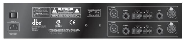
**Power Switch:** Switches the power on and off. Always make audio connections with the power switch in the OFF position.
