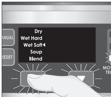
2. Press Process Selection Button until arrow reaches desired operation. Each operation has a set blending time.
