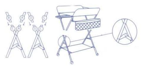
Connect the upper and lower components installed in Step 1 according to the corresponding letter labels
