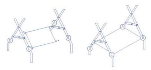
The steel price side with the letter label faces outward, and the long steel pipe is connected to B and C, and the short pipe is connected to A and D
