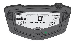
Once the cluster is connected with the smart phone, the cluster displays the signal strength of the network provider 'Till' and the battery level 'III' of the smart phone. Number of unread messages 'III' and number of missed calls 'III'.
