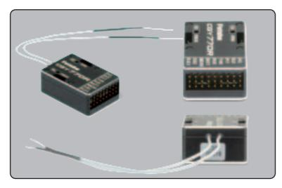
Futaba CGY770R is gyro, 3-axis Stabilization System combining AVCS gyro and head speed governor and receiver in one box designed for flybarless helicopters. Its cutting edge MEMS (Micro Electro Mechanical System) sensor design, ultra high-speed processing speed, and advanced PID control algorithm put it a league of it's own ahead of all ahead of all other heading hold gyros in size, weight and performance.
