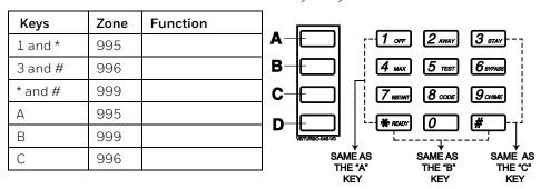
To use a paired key panic function, simply press both keys of the assigned pair at the same time.
