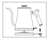
Step 2. Put the lid on the pot and place the pot on the power base. Pay attention to good contact.please do not exceed the maximum water level.
