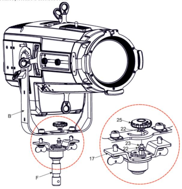
7.1 Insert the spigot (F) with adaptor (17) to the tripod. The opening (18) has to be oriented as shown on the picture.
