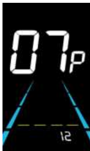
Number of speed sensor magnets setting
