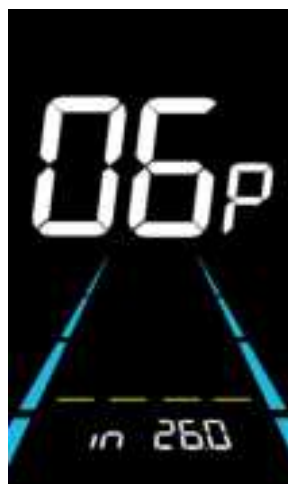
Wheel diameter setting interface
