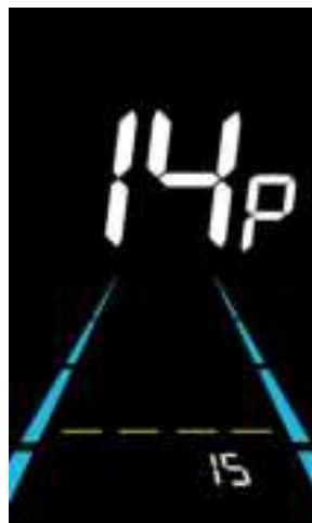
Controller current limit setting interface
