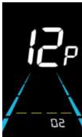
Pedal assist Start-up intensity interface
