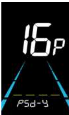
Power-on Password Activated interface
