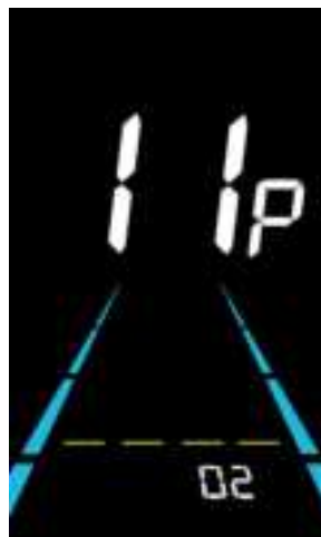
Pedal assist sensitivity setting interface
