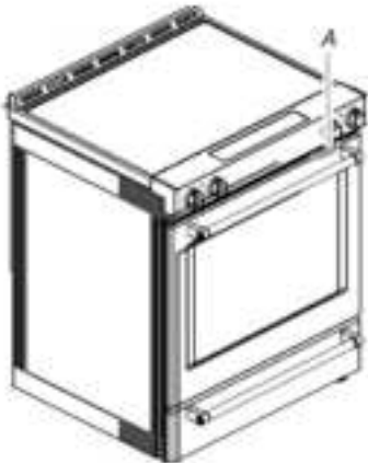
A. Model/serial/rating plate (located behind the oven door on the top right-hand side of the oven frame)
