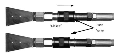
♦ Position the Turbo Blast Nozzle to the direct air towards the Rim Center just under the Rim Lip.
