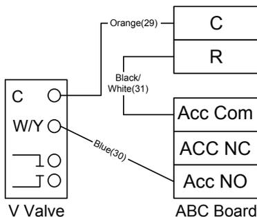
**NOTE:** SW2-4 should be "ON" and SW2-5 should be "OFF" when using a slow opening (V100FPT) water valve.
