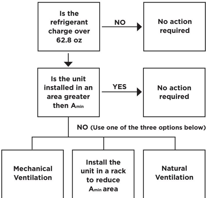
Use Table 1 to determine the minimum floor area,  $A_{min}$ . The equipment must be installed with a minimum floor area equal to or larger than the area listed in the chart based on the total refrigerant charge of that system. If the area is not large enough, you must move to the next step for additional installation requirements.
