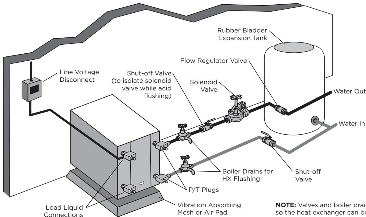
**NOTE: Valves and boiler drains must be installed so the heat exchanger can be acid flushed.**
