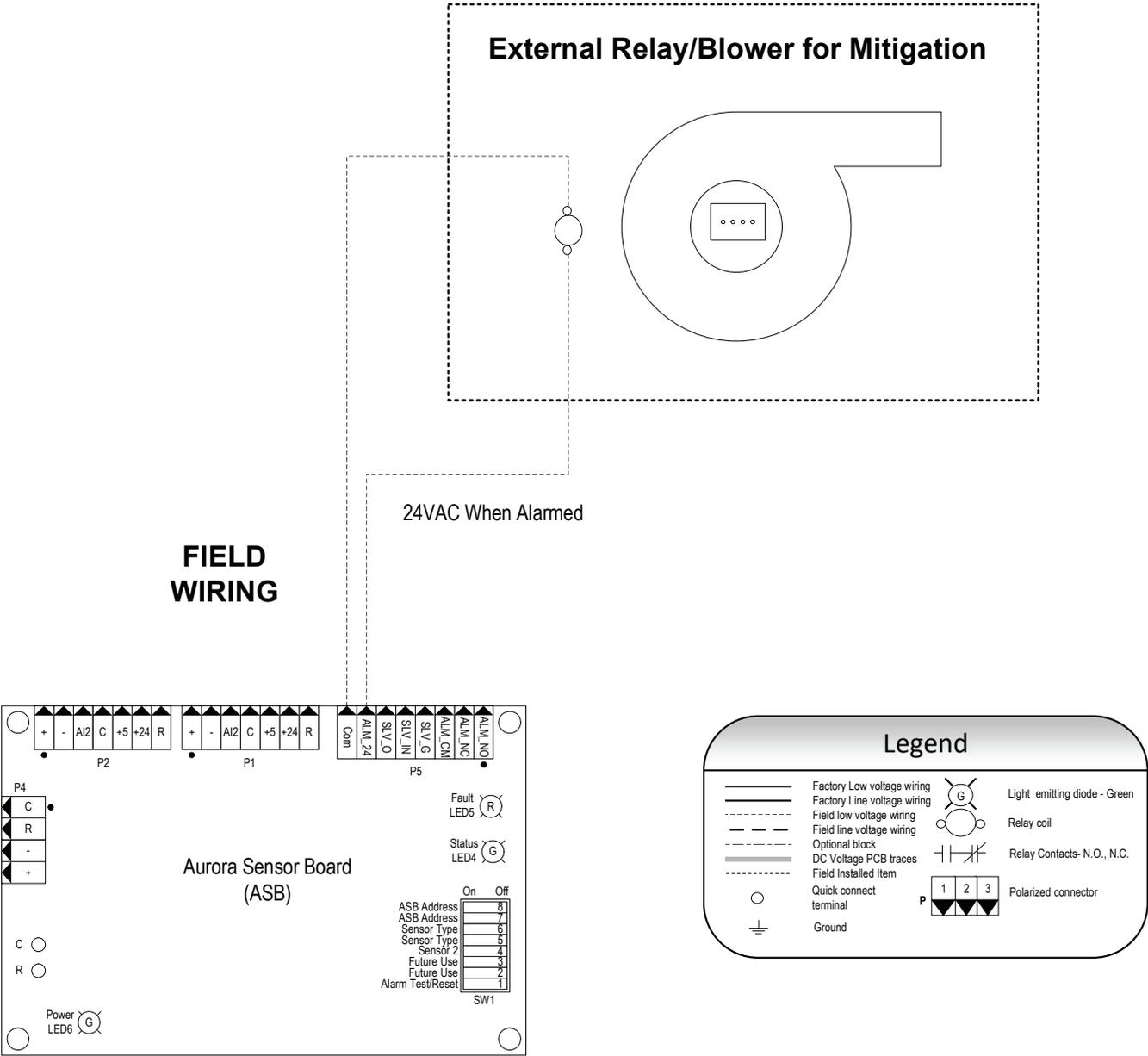
Figure C: Refrigeration Detection and Mitigation Wiring Example
