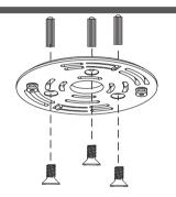
Use the included hardware to attach the mounting plate to the ceiling as shown. Point the arrow on the mounting plate in the direction you want the camera to face.
