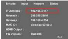
(2) Open the browser and input the IP address, e.g. 192.168.4.147, to access the login interface.
