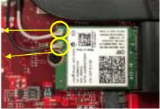
⚠ After the WIFI card is assembled, please paste the CABLE TAPE and Mylar according to the following positions.
