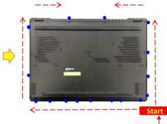
▲ Please follow above arrow direction with using plastic blade to pry bottom case in each blue circle location.(To avoid the bottom case hook, please prying at each blue circle location.)
