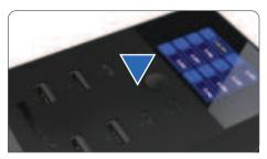
3. Activate the screen by pressing and holding down the function button for 2 full seconds. You may then review the power status of all 8 ports and cycle to see per-port details for voltage, amperage, temperature, and charge time.
