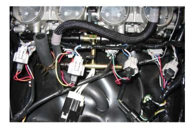
6 Attach the connectors from the PC6 to the stock wiring harness and the throttle bodies as shown.
