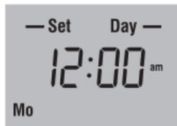
**NOTE:** *The clock has lost its settings when the time display flashes. If the thermostat is following the schedule, it will use the temperature settings programmed for the Wake period of the weekdays until you readjust the clock.*
