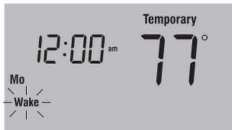
**NOTE:** Pressing the **Up** or **Down** button once will display the setpoint temperature. To change the setpoint temperature, press either button more than once.
