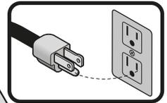
**⚠ WARNING** When using an extension cord, make sure to use the proper gauge to carry the current your tool will consume. An undersized cord will cause voltage drops in the line, resulting in power loss and motor overheating. The following table shows the correct size to be used depending on the cord length and the amperage capacity indicated on the tool's data plate. If in doubt, use the next higher gauge.
