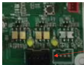
15V Input Power on Inverter PCB.
