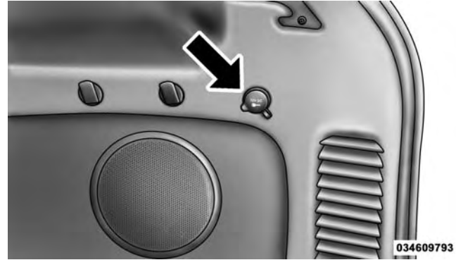
Rear Power Outlet
