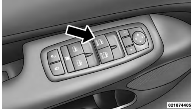
Auto-Down Window Switches
