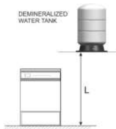
Fig. 4 – Unpressurised tank, height above device installation surface L > 100 \text{ cm} .
