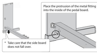
2. Align the screw holes of the metal fitting with the screw holes of the pedal board, and provisionally hand-tighten the large screw **9**.
