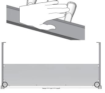
8. From the back of the rear board, use pointed screws (four locations).
