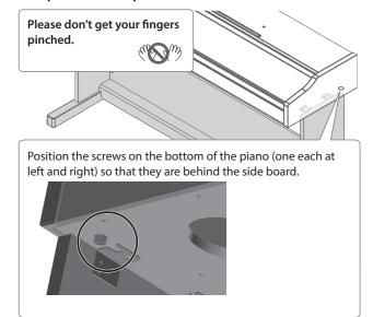
**2.** Align the screws on the bottom of the piano with the metal fittings of the side board.
