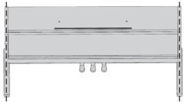
5. Install the two large screws in the bottom of the piano. First use your hand to tighten the large screws
