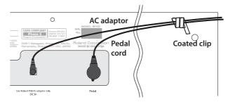
**10.** Connect the supplied AC adaptor and power cord, and plug the power cord into an AC outlet.
