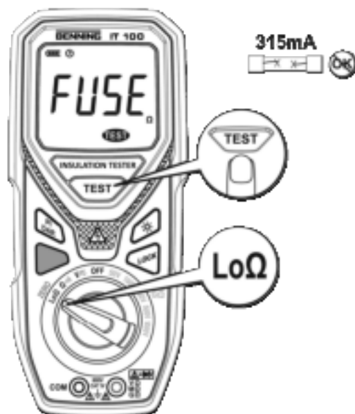
Figure 12: Testing the fuse
