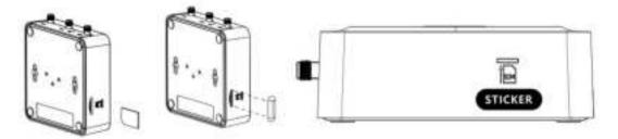
2. Antenna Installation. Rotate the antenna into the antenna connector accordingly.
