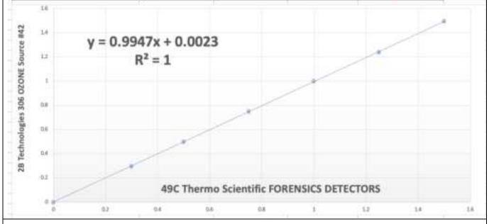
Based on the following unbroken chain of comparisons that are based on the US National Institute of Standard and Technology (NIST), FORENSICS DETECTORS calibrates all of its sold ozone meters, detectors, analyzers and monitors to either:
