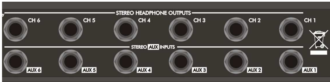
FIGURE 3 - Rear Panel Headphone Outputs and Aux Inputs
