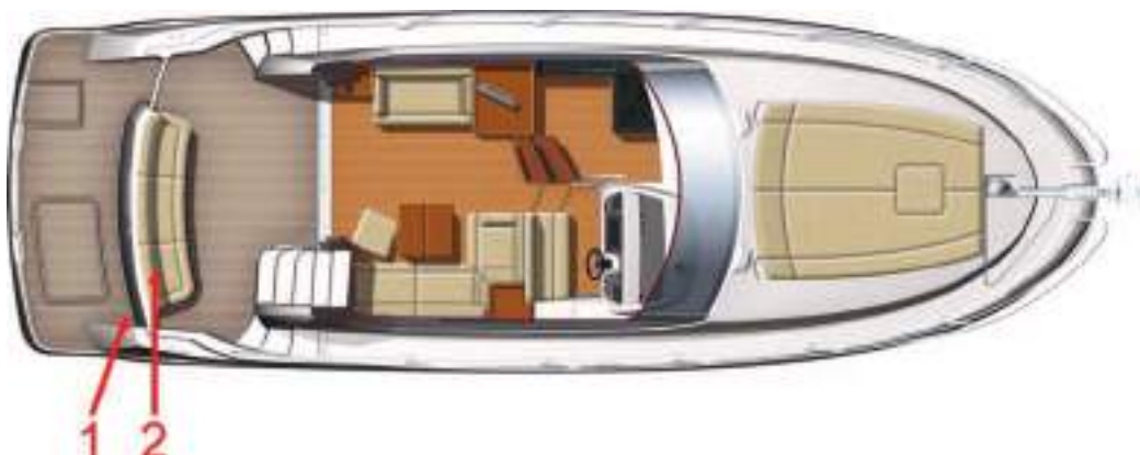
Shore power socket 220V - 32A (Reference 1)
