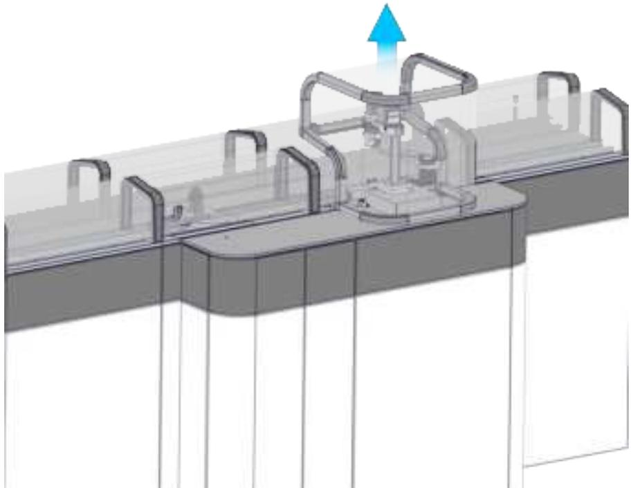
3. Pull up the Decapper head and rotate it to the decap position by hand.
