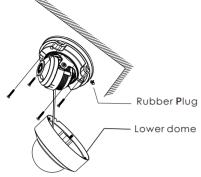
(6) Three-axis adjustment. Before adjustment, view the image of the camera on a monitor and then adjust the camera according to the figure below to get an optimum angle.
