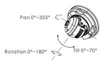
① Install the lower dome back to the camera and fix it with the screws. Then put the trim ring onto the lower dome and then rotate it clockwise until it is locked.
