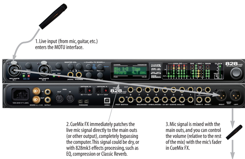
Figure 9-2: This diagram shows the signal flow when using CueMix FX no-latency monitoring. Notice that this method does not process the live input with plug-ins in your audio software. Instead, you can apply 828mk3 effects, such as the reverb, EQ and/or compression.
