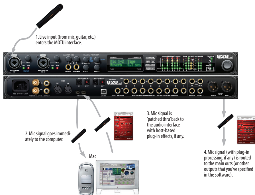
Figure 9-1: There are two ways to monitor live audio inputs with an 828mk3: 1) through the computer or 2) via CueMix FX hardware monitoring. This diagram shows method 1 (through the computer). When using this method, use your host software's buffer setting to reduce the slight delay you hear when monitoring the live input, but don't lower it too much, or your computer might get sluggish.
