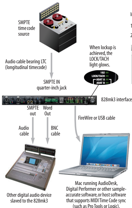
Figure 3-17: Connections for synchronizing the 828mk3 directly to SMPTE timecode.
