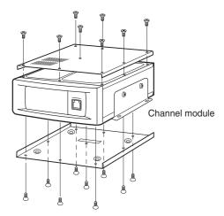
② Re-install the channel module and the screws to their original positions, and then connect the control cable of the repeater's front panel to the channel module.
