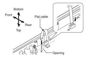
② Turn over the channel module. Carefully pull out the other end of the flat cable from the opening, and then insert it into J1 on the
