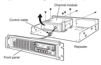
③ Unscrew the eight screws from the top, the nine screws from bottom, and the three screws from rear of the channel module. Then remove each cover from it.
