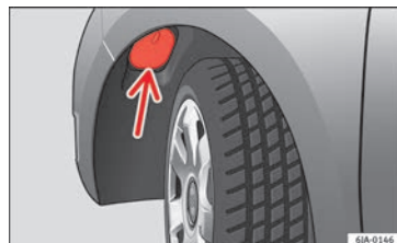
Fig. 91 Changing dipped beam headlight bulbs: wheel housing.
