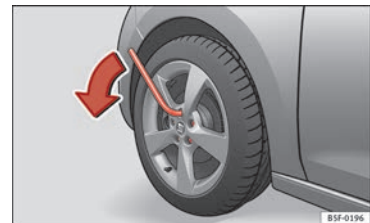
Fig. 62 Changing a wheel: loosen the wheel bolts.
