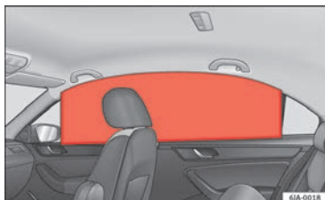
Fig. 21 Deployed head-protection airbags.
