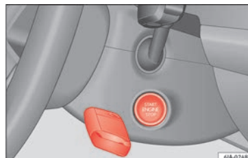
Fig. 174 Emergency ignition in vehicles with Keyless Access.
