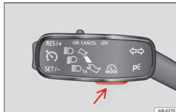
Fig. 191 On the turn signal and main beam headlight lever: button for the driver assistance systems
